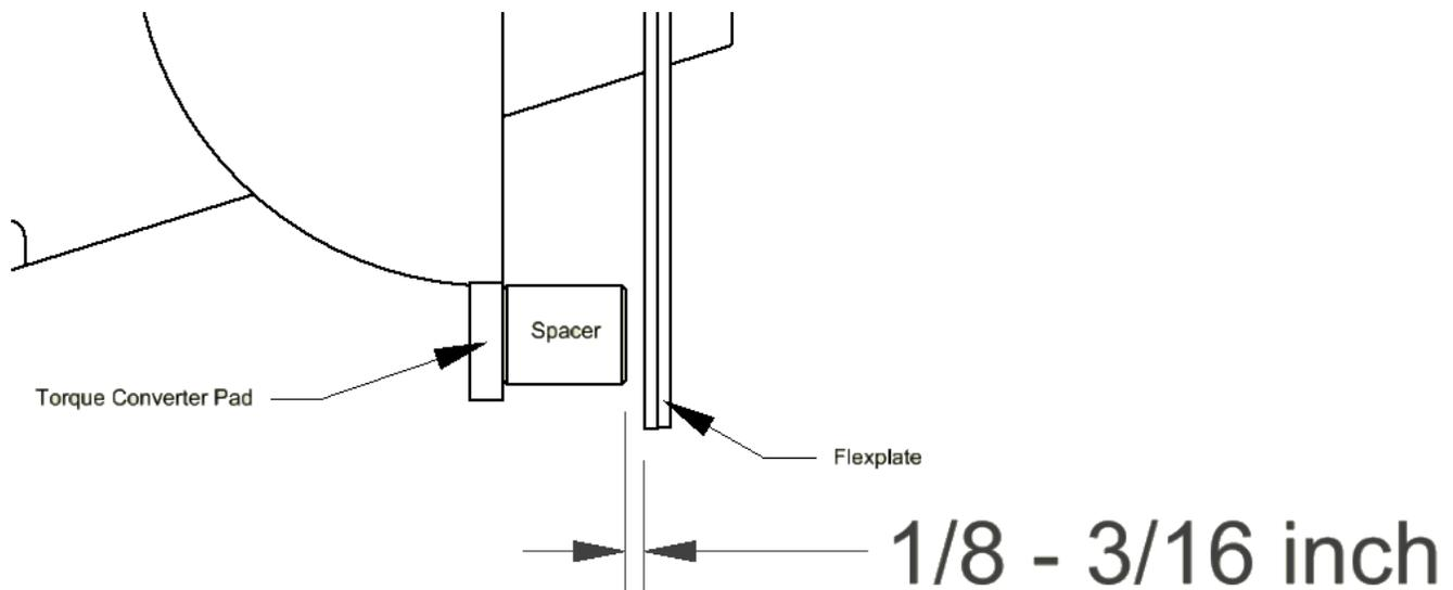
8. Bolt torque converter to flexplate **WITH SPACERS INSTALLED BETWEEN FLEXPLATE AND TORQUE CONVERTER**. Apply locking compound to the threads and torque bolts to **58 ft-lbs**. Some kits do not need spacers. Verify that the gap distance is correct for your application.
