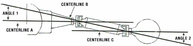
In the diagram, Angle 1 is defined as the intersecting angle between the centerline of your transmission output shaft and the centerline of the driveshaft. Angle 2 is defined as the intersecting angle between the centerline of the driveshaft and the center line of your pinion.
