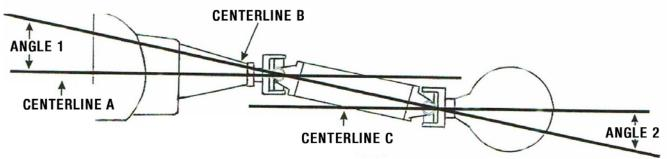
TCI<sup>®</sup> Automotive 151 Industrial Dr. Ashland, MS 38603 Phone: 662.224.8972 In the diagram, Angle 1 is defined as the intersecting angle between the centerline of your transmission output shaft and the centerline of the driveshaft. Angle 2 is defined as the intersecting angle between the centerline of the driveshaft and the center line of your pinion.
